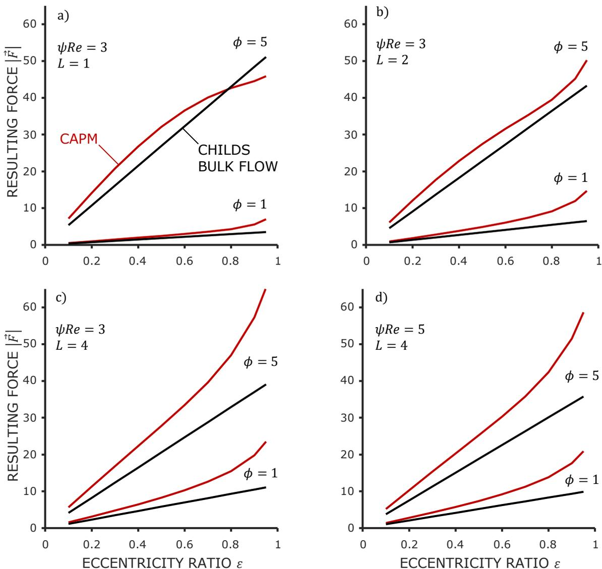
Figure 5. Comparison of force over eccentricity for the CAPM and the bulk flow model. Diagrams a), b) and c) show results for  $\psi Re = 3$  and  $L = 1, 2, 4$ . Diagram d) shows results for  $\psi Re = 5$  and  $L = 4$ .
