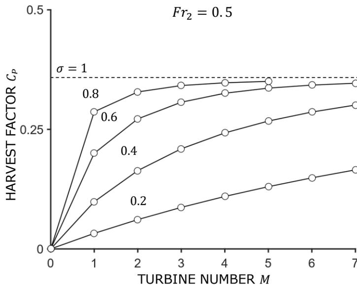
Fig. 5: Harvest factors for turbine cascades of up to seven turbines for an exemplary Froude number of  $Fr_2 = 0.5$ .
