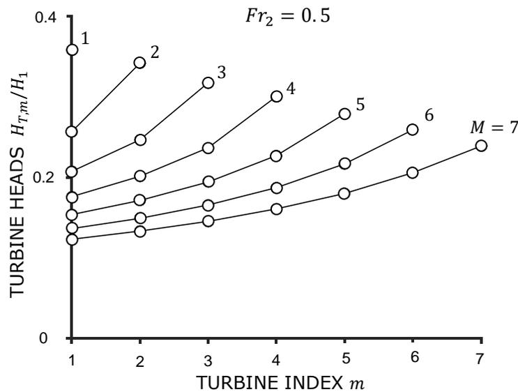
Fig. 6: Harvest Factors for turbine cascades of up to seven turbines for an exemplary Froude number of  $Fr_2 = 0.5$ .
