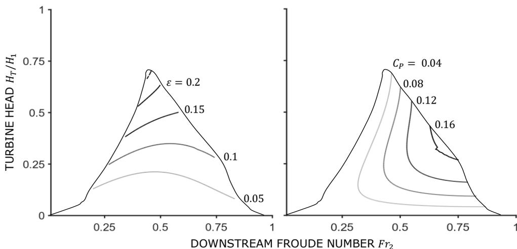
Fig. 2: mixing inefficiency  $\varepsilon$  and harvest factor  $C_p$  as a function of turbine head  $H_T$  and downstream Froude Number  $Fr_2$  for a single turbine with exemplary blockage of  $\sigma = 0.4$ .
