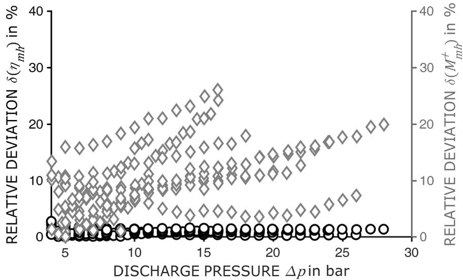
Figure 5: Relative deviation of the friction torque model (grey diamond marker) and the mechanical-hydraulic efficiency model (black circle marker) versus the discharge pressure.
