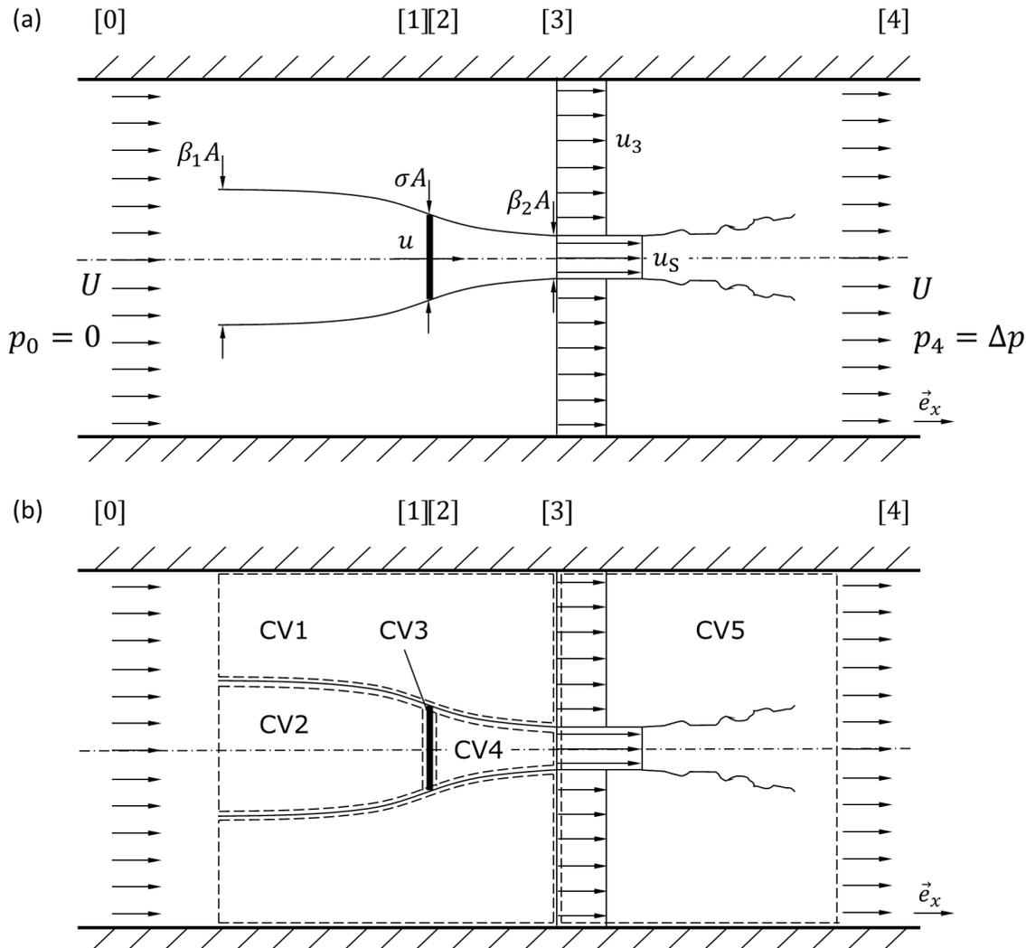
Figure 2: Schematic sketch of one ventilation unit: (a) velocities and cross sections. (b) Control volumes (CV).
