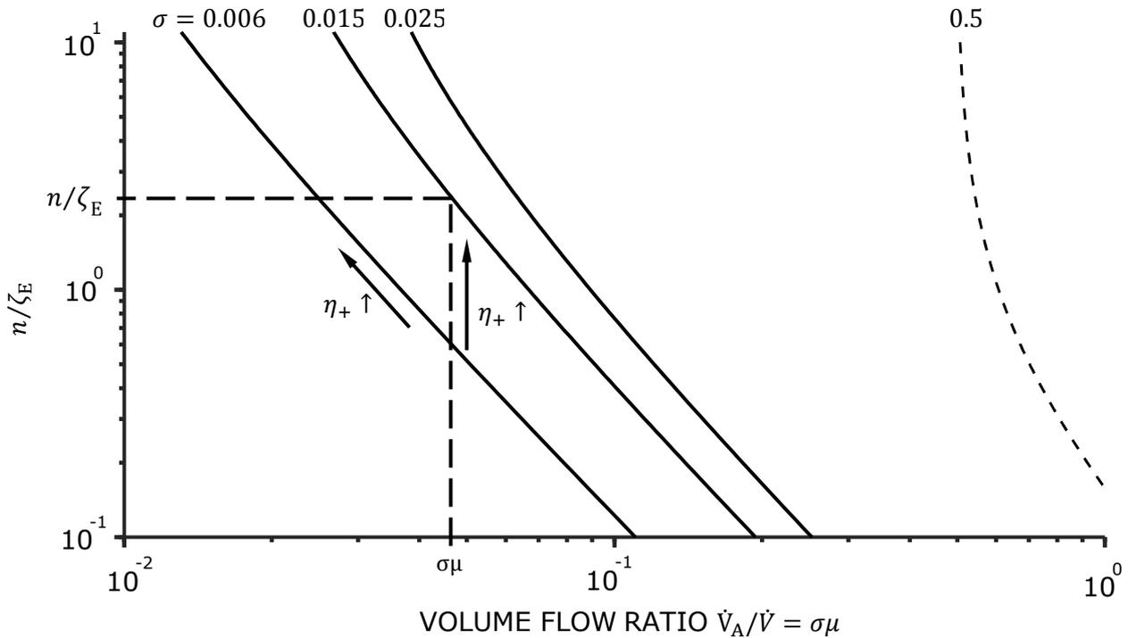
Figure 8: Number of jet fan units per loss coefficient  $n/\zeta_E$  versus volume flow ratio  $\dot{V}_A/\dot{V} = \sigma\mu$  with the cross section ratio  $\sigma$  as independent variables.
