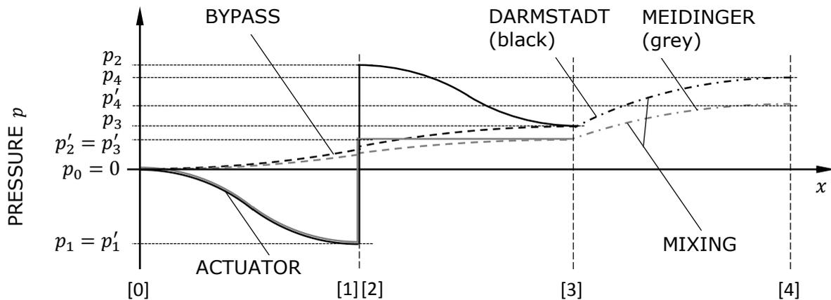
Figure 9: Qualitative characteristic of static pressure through the tunnel ventilation unit.
