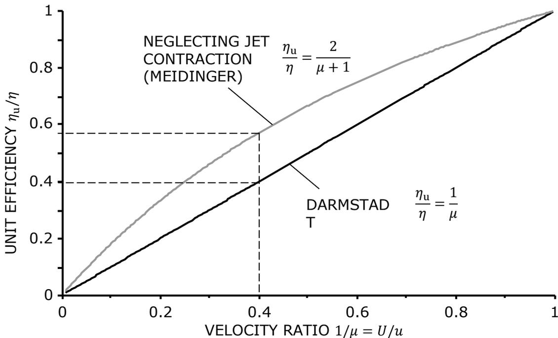
Figure 6: Unit efficiency  $\eta_u$  versus the velocity ratio  $\mu$  for Meidinger’s and Darmstadt’s method for all cross section ratios  $\sigma$ .
