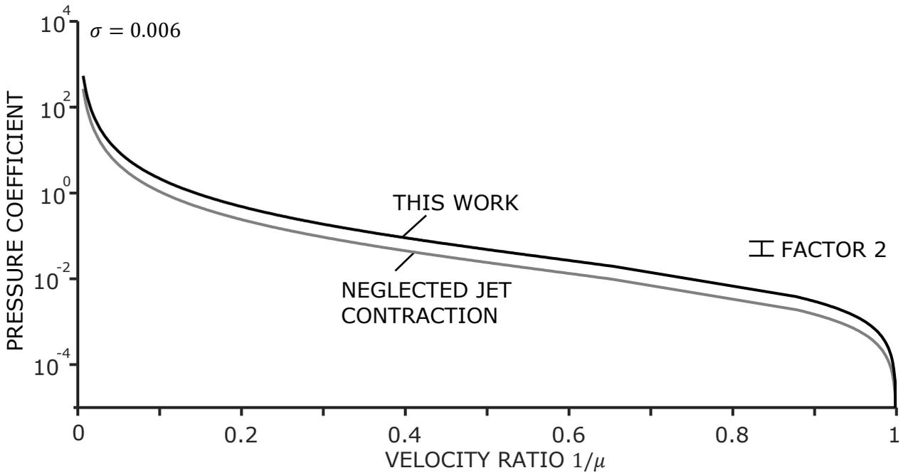
Figure 5: Comparison of total pressure rise  $\psi$  versus velocity ratio  $\mu$  between the presented model and Meidinger's model. This model takes the contraction of the stream tube into account.
