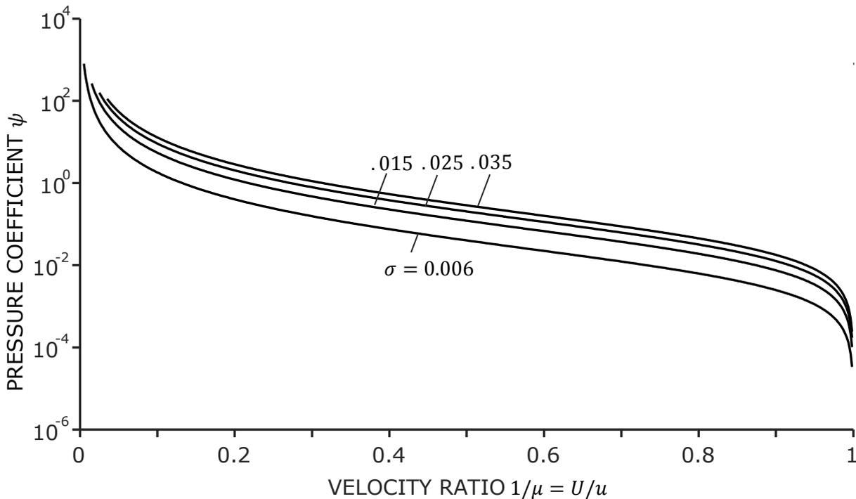
Figure 4: Pressure rise  $\psi$  versus velocity ratio  $\mu$  for changing area ratios  $\sigma$ .
