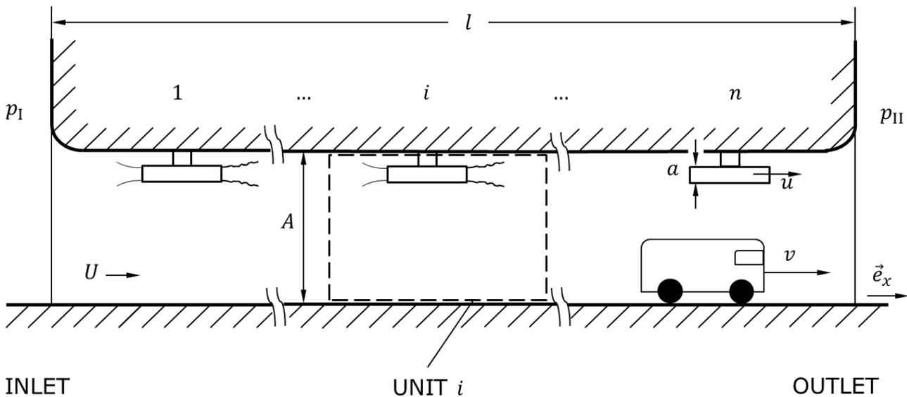
Figure 1: Tunnel ventilation system with jet fans and traffic.
