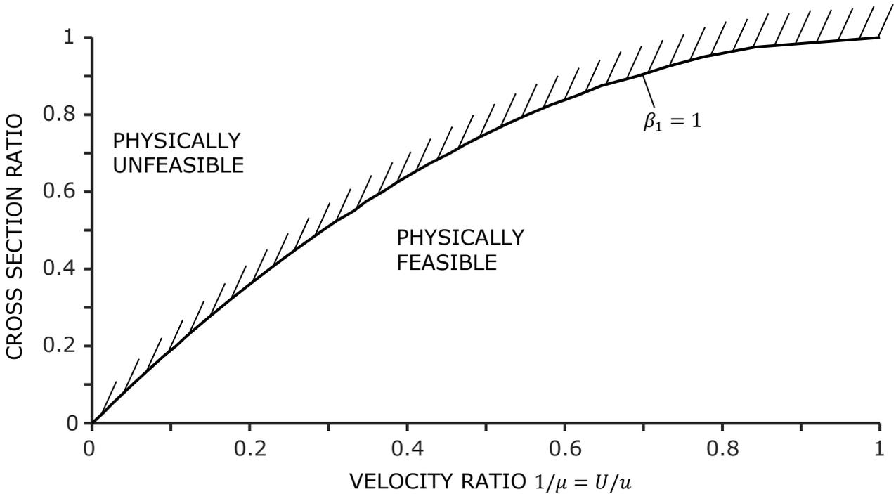
Figure 3: Physically feasible und unfeasible combinations of cross section ratio  $\sigma$  and velocity ratio  $1/\mu$ . Please note, typical cross section ratios for tunnel ventilation are  $\sigma = 0.005 \dots 0.02$  and the velocity ratio is  $1/\mu \approx 0.17$ .
