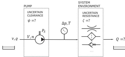
Figure 3: Schematic view of a generic fluid system.
