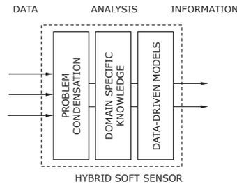
Figure 1: "Filter disks" of a hybrid soft sensor.
