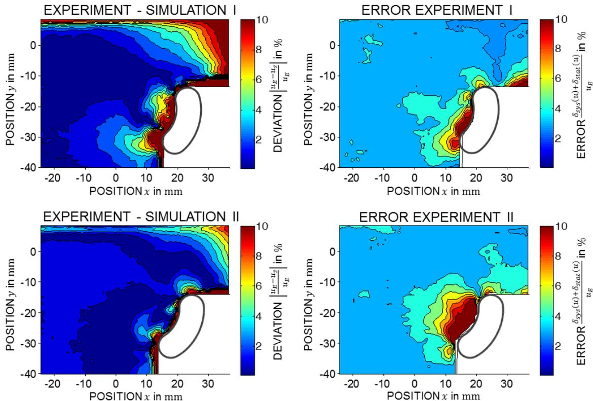
Figure 2: Left side, relative deviation between experiment and simulation for configuration I ( $\bar{U} = 15$  m/s,  $\alpha = 45^\circ$ ) and II ( $\bar{U} = 20$  m/s,  $\alpha = 30^\circ$ ). Right side, relative measuring error of configuration I and II.
