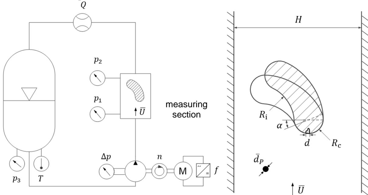
Figure 1: Hydraulic diagram of the Test Rig with sensors and sectional drawing of the measuring section. The absolute pressure in the pressure vessel  $p_3$  and measuring section ( $p_1, p_2$ ), the differential pressure across the pump  $\Delta p$ , the temperature  $T$ , the volume flow  $Q$ , the rotational speed of the pump  $n$  and the frequency of the frequency converter  $f$  are measured during a quasi-stationary operating point.
