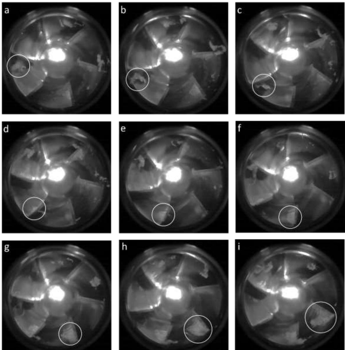
Figure 7: Formation of sheet cavitation due to gap cavitation. The time interval between the images is 2 ms.  $q = 0.4$ ,  $n = 1750$  rpm,  $NPSH = 2.50$  m, rough leading edge 3 mm,  $k = 52$   $\mu$ m.
