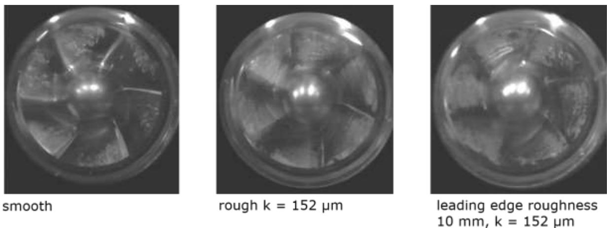
Figure 5: High-speed visualization (exposure time 0.2 ms) of impeller with different roughnesses (cf. figure 3) in the same operation point.  $q = 0.8$ ,  $n = 1750 \text{ rpm}$ ,  $\text{NPSH} = 1.50 \text{ m}$ .
