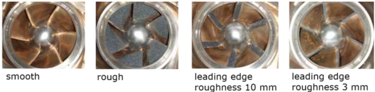
Figure 3: Measured roughness configurations.
