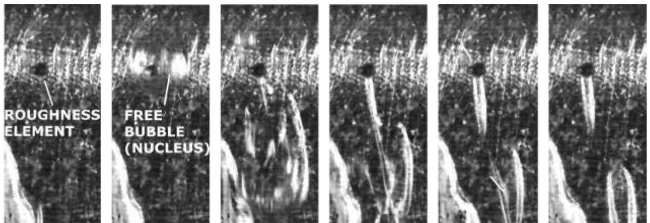
*Figure 8: High-Speed visualization of the activation of a roughness element. The flow is from top to bottom. The time interval between the images is 0.2 ms. The roughness element has got a diameter of 0.1 to 0.15 mm.*
