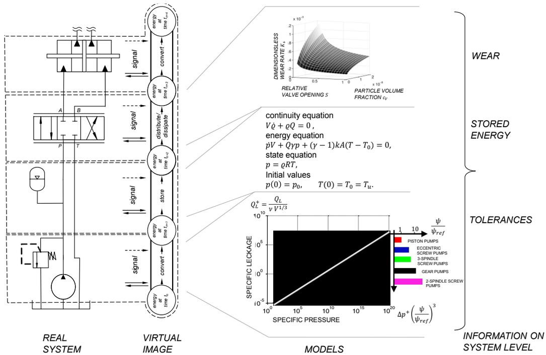
**Fig 3** Soft sensor network of a hydraulic drive system
