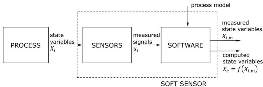
**Fig. 1** Generic functional principle of a soft sensor
