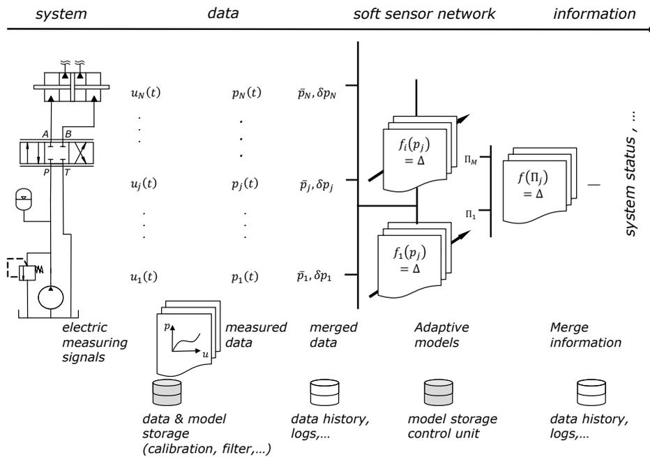
Fig. 2 Generic approach to aggregate system information based of a soft sensor network
