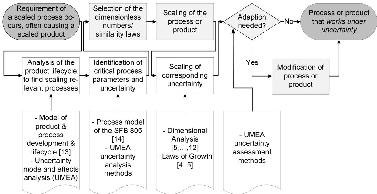
Figure 1: A procedural model of the scaling process, including the analysis and assessment of uncertainty. The light grey processes are also part of the scaling process without considering uncertainty. Supporting methods are displayed in the third row of the diagram.
