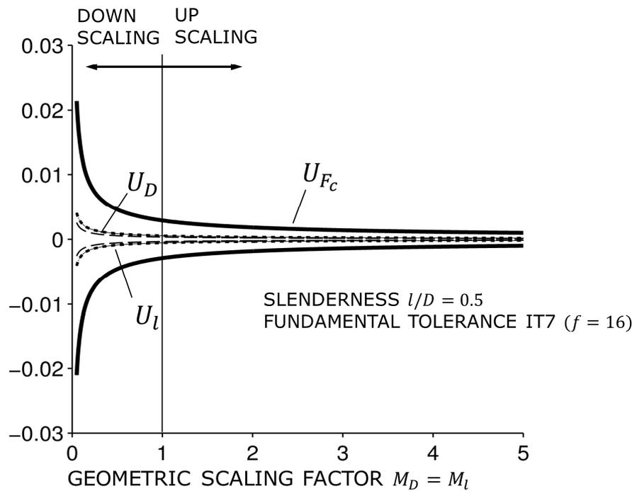
Figure 5: Uncertainty of the geometric values and the critical buckling load of the beam.
