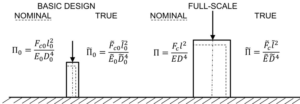
Figure 4: Nominal and true values of the basic design and a geometric scale of a buckling beam.
