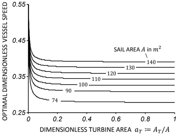
Figure 3: Optimal vessel speed for varying sail areas.
