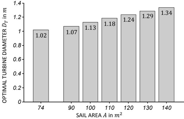
Figure 6: Optimal turbine diameter for varying sail areas.
