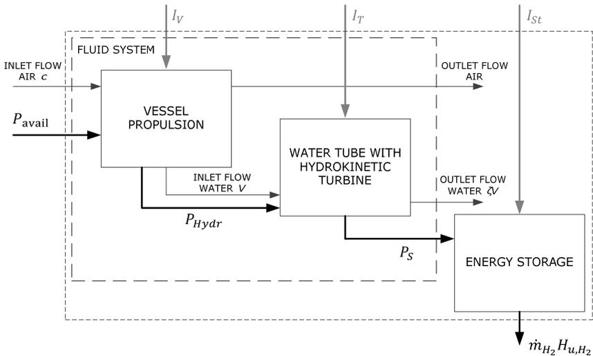
Figure 1: Block diagram of the energy ship.
