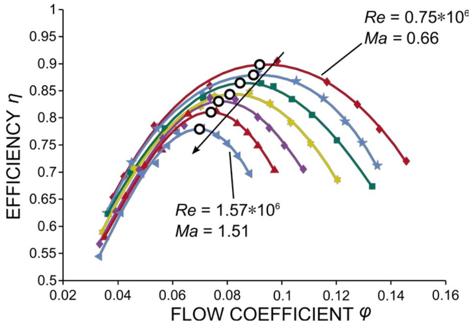
Figure 1: Measured efficiency versus flow coefficient for a compressor with Reynolds and Mach number varied. Peak efficiencies are marked by a circle. They are all aligned along a straight line [7].
