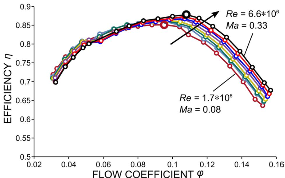
Figure 2: Variation of the best efficiency point of a centrifugal fan [6].
