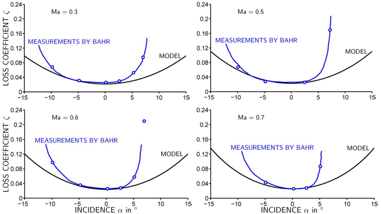
Figure 7: Comparison of the model and validation data at  $Re = 2 * 10^5$  and a solidity of  $l/t = 1$ .
