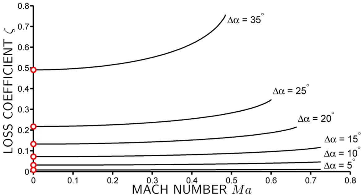
Figure 4: Incidence loss for compressible flows
