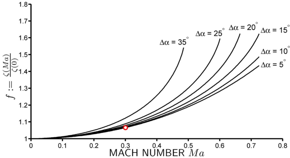
Figure 5: Correction function for the incidence loss
