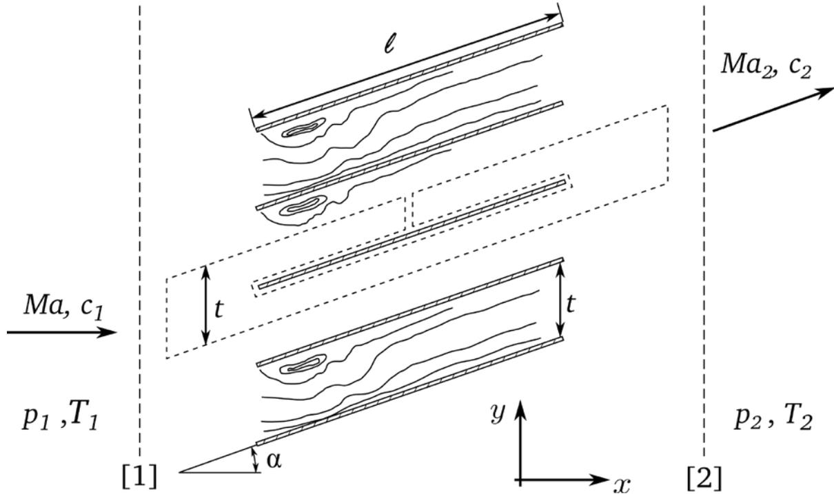
Figure 3: Schematic flow through a cascade of flat plates.
