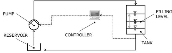
We model this setup by a mathematical graph  $G = (V, E)$ . The reservoir and the tank are represented by vertices  $V$ , pumps and pipes by edges  $E$ . The following physical equations and models describe the filling level system and are included into the MILP formulation. First, the continuity equation for incompressible fluids results in the conservation of volume flows  $Q$ .
