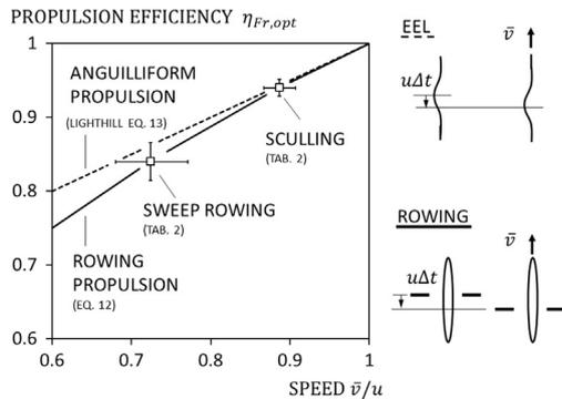
Fig. 4. Upper limit for the efficiency of any paddling or rowing motion in comparison with anguilliform propulsion.
