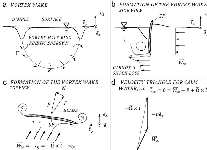
Fig. 3. (a) Vortex wake of the blade; (b) and (c) Formation of the vortex wake; and (d) Velocity triangle (outboard length  $l$ ).
