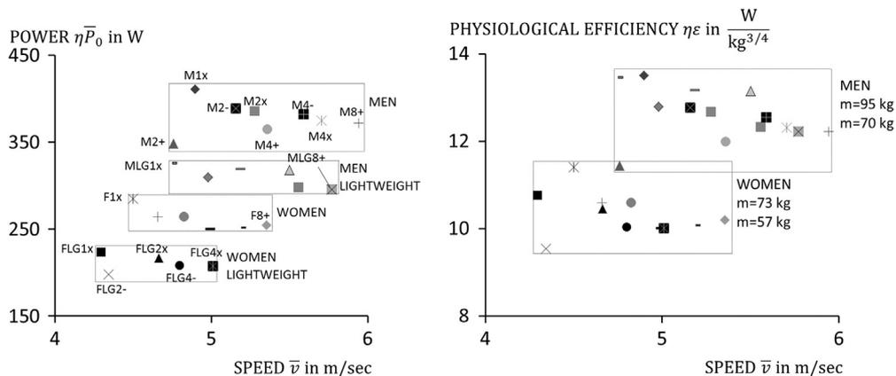
Fig. 5. Transmitted power per rower versus boat speed (left) and the product of physiological efficiency and efficiency vs. boat speed (right), as determined using Eq. (14). Data comes from the winning crews in the Olympic, World Rowing Championship and Luzern International regattas in the decade from 1997 to 2007. The left diagram shows the validity of allometric scaling for competitive rowers.
