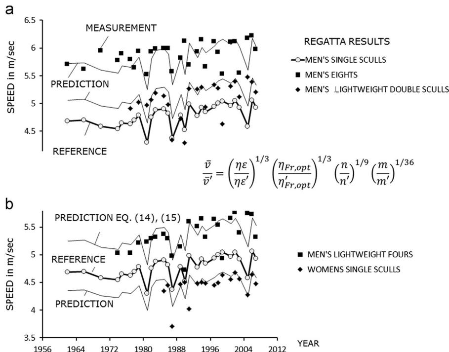
**Fig. 6.** Validation of the scaled speed of rowing (Eq. (14)) using measured winning race speeds. Reference is the men's single sculls result (thick solid line).
