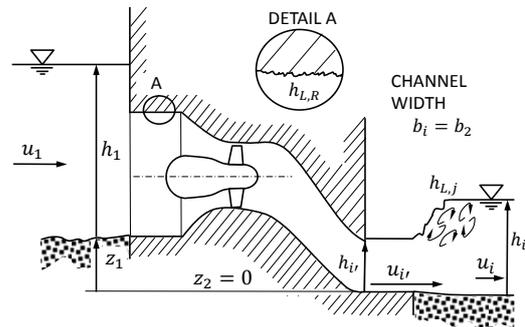
Figure 5: Draft tube without diffuser (Case I)
