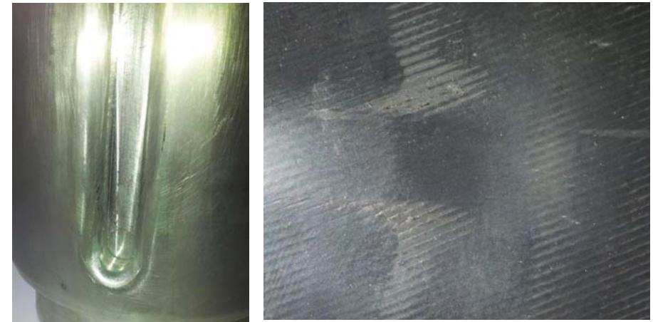
Figure 2: Passive piston with the active pistons geometry (left), abrasive damage to the bellows (right)
