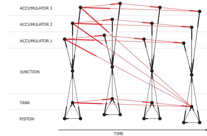
Figure 4: Mathematical graph of the hydrostatic power transmission system
