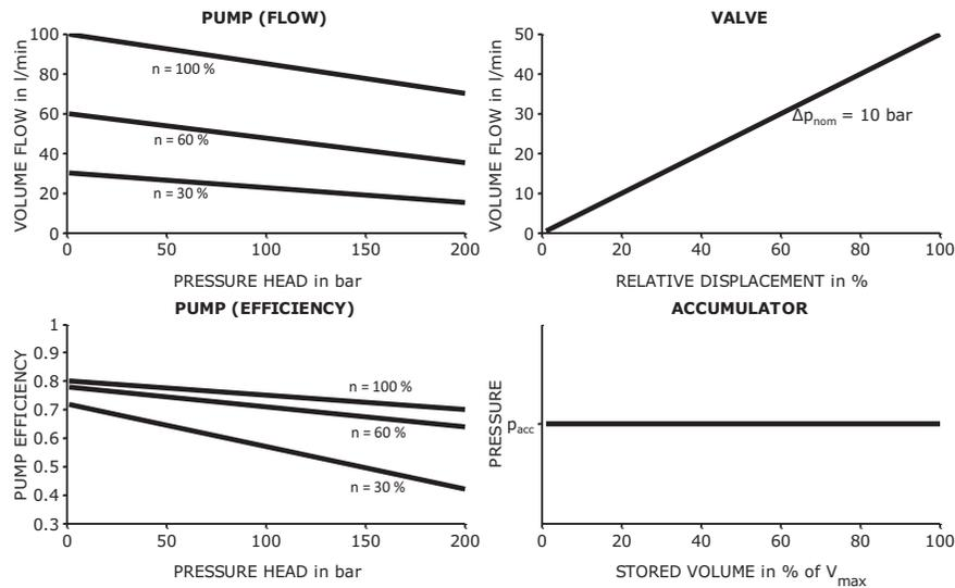
Figure 3: Characteristic curves of the construction set
