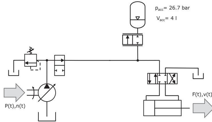
Figure 6: Topology of the optimal System designed by TOR
