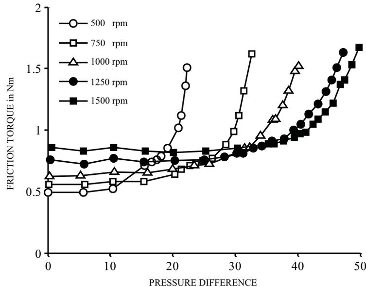
*Figure 4: Measured friction torque for a three spindle screw pump.*
