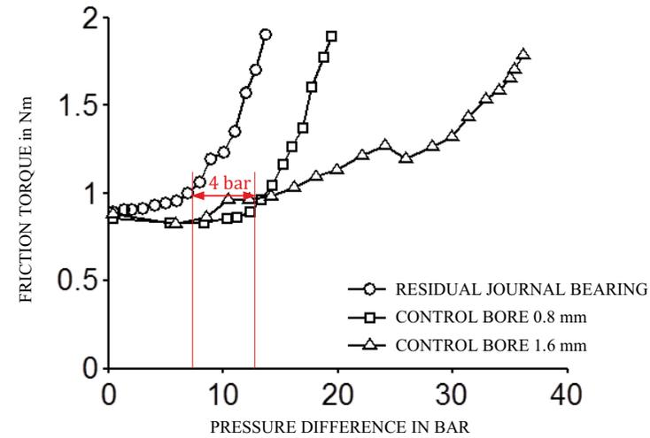
Figure 11 Friction torque of the modified screw with and without compensation system as 1500 rpm.
