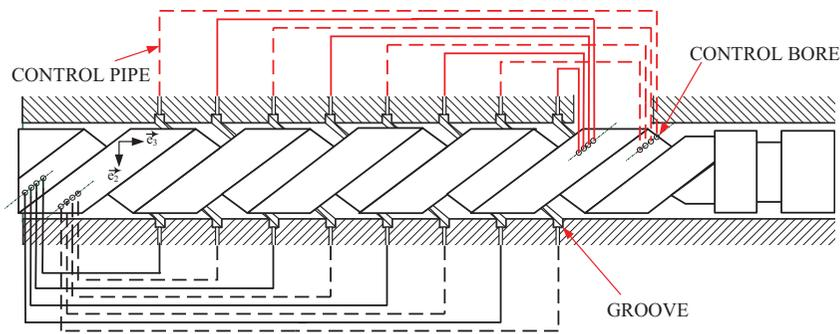
Figure 6 Hydraulic wiring scheme of the compensation system.
