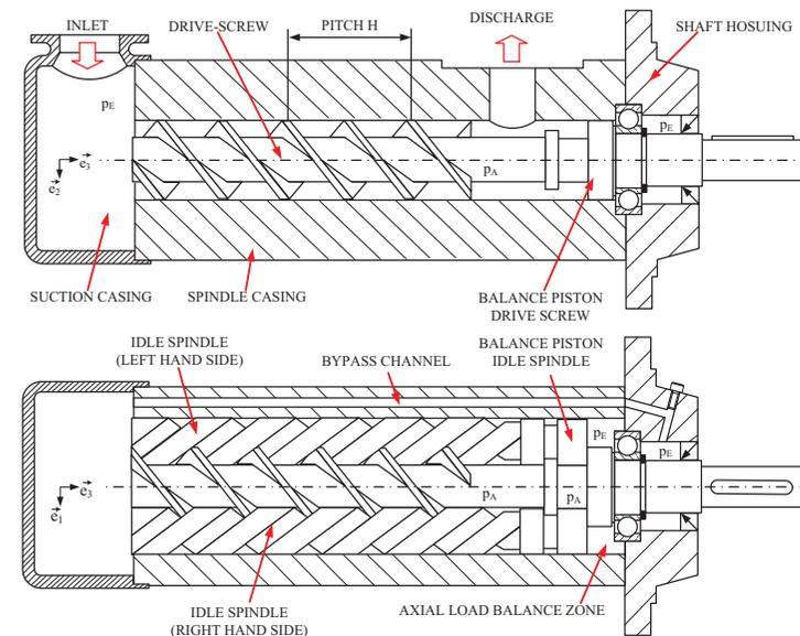
Figure 1: Setup of the three spindle screw pump.
