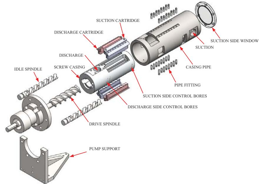
Figure 7 Exploded assembly drawing of the screw pump with the added compensation system.
