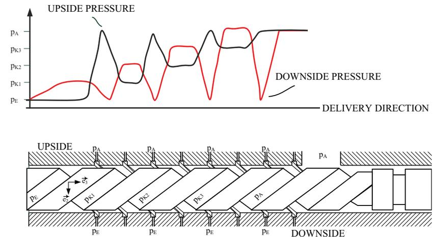
*Figure 5 Concept of the lateral load balancing at the right idle spindle.*
