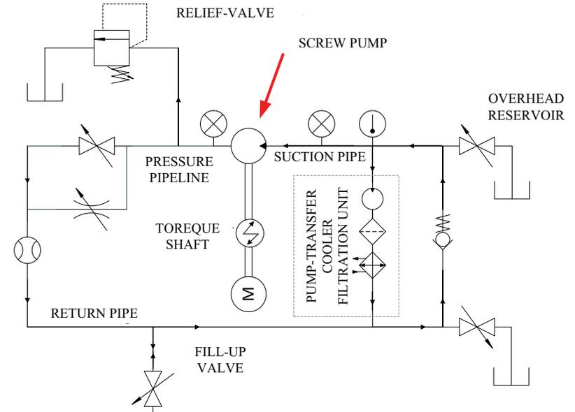
Figure 3: Hydraulic wiring scheme of the test rig.
