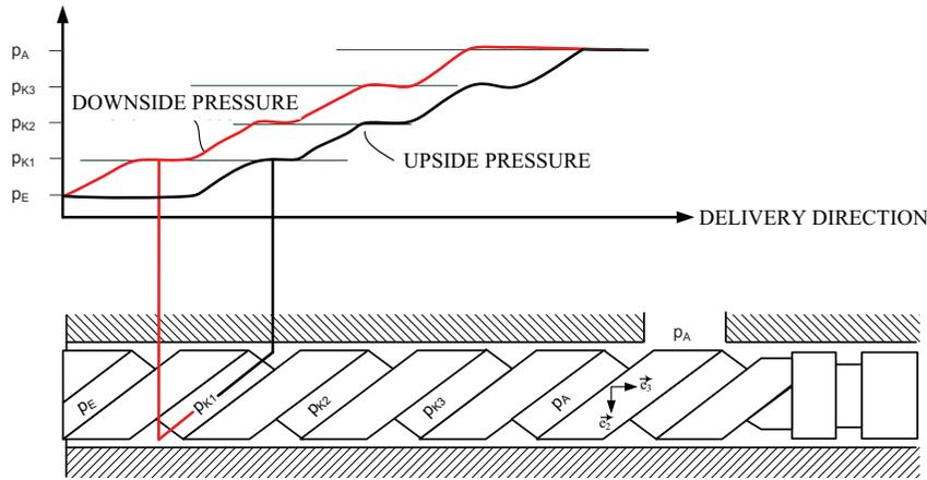
Figure 2: Sketch of the hydrostatic load across right idle spindle.
