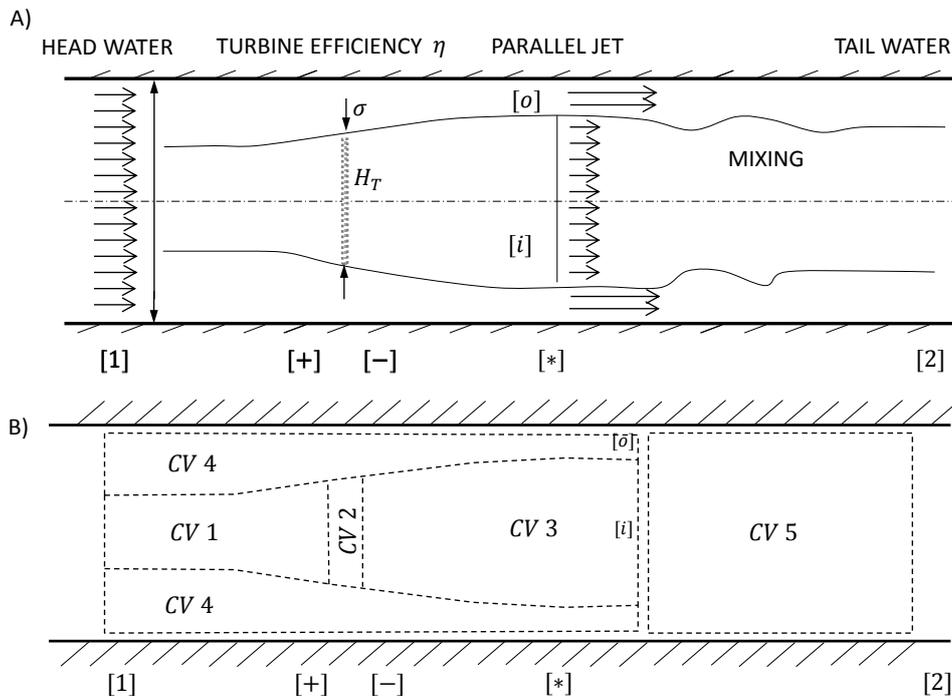
Fig. 3: 0-dimensional disc-actuator model for tidal turbines
