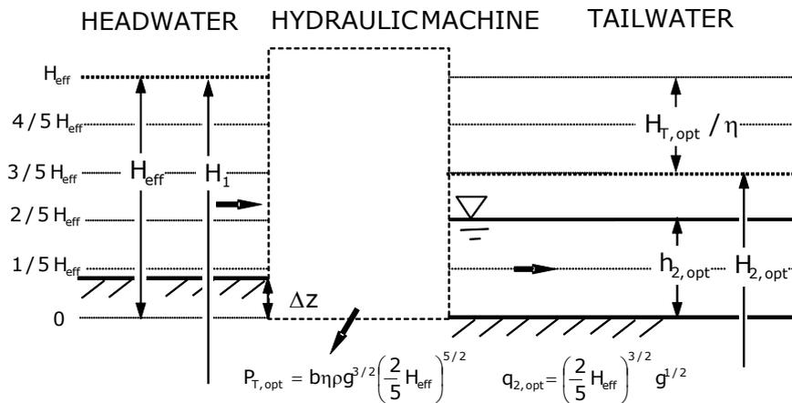
Fig. 1: Optimal operating point for hydropower [1].
