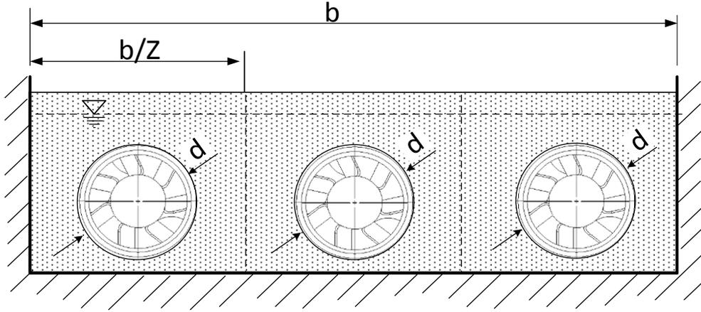
**Fig. 5:** Cross section through transverse structure of hydro energy plant with  $Z=3$  modules.
