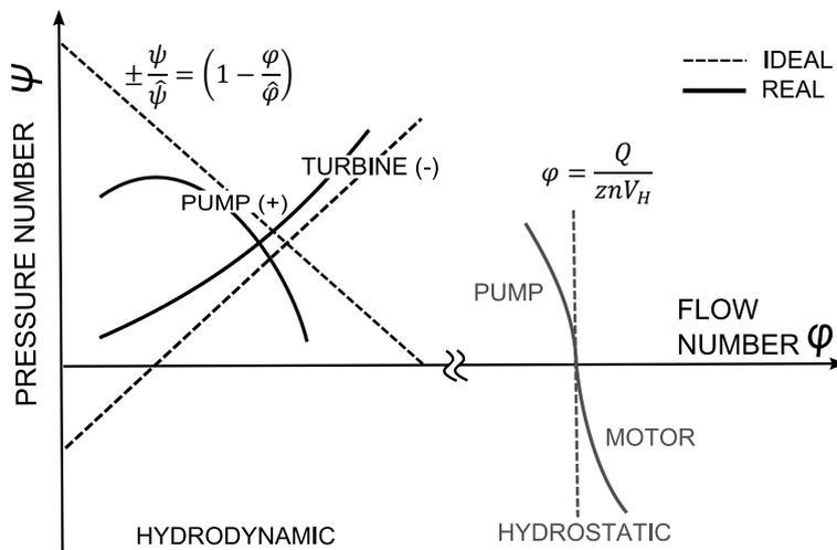
**Fig. 4:** Characteristics of pumps and turbines/motors.
