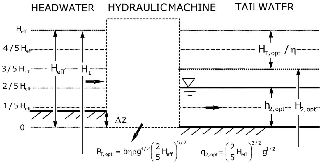
Fig. 1: Optimal operating point for hydropower [7].
