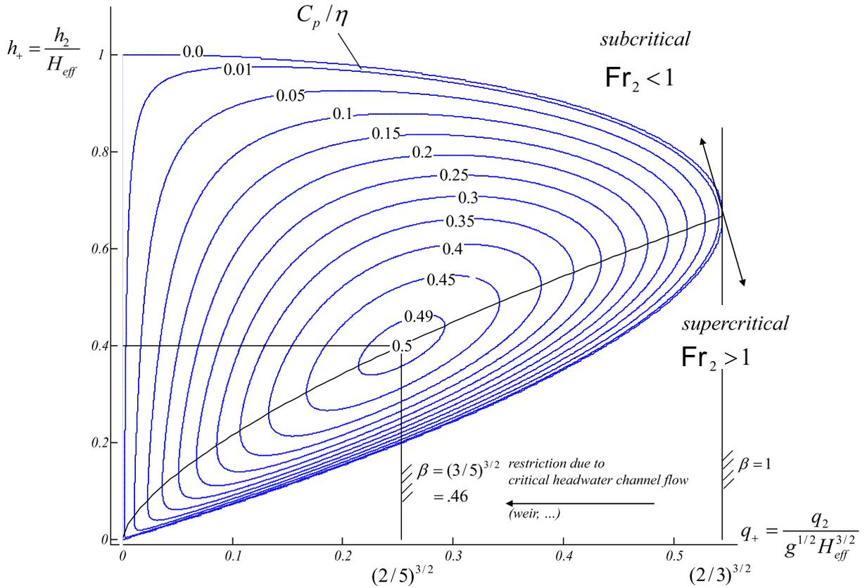
**Fig. 2:** Coefficient of performance as a function of dimensionless volume flow rate and head [7].
