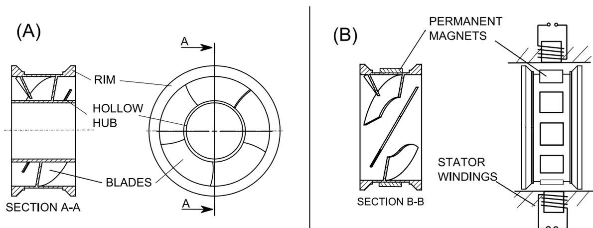
Fig. 6: Design of a fish friendly turbine [8].
