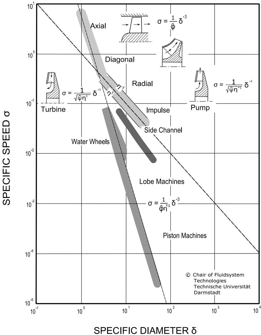
Fig. 3: Corider-diagram with machine typology and asymptotes.
