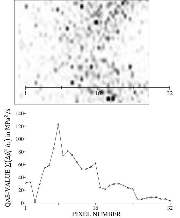
**Fig. 6:** Comparison of damage map (Pit-Count measurement from [1], upper half of figure) and quadratic amplitude sum determined from measured signals of one pixel line of sensor prototype (lower half of figure) for operating point  $\sigma = 5.45$  and  $Re = 2.75 \times 10^5$ .
