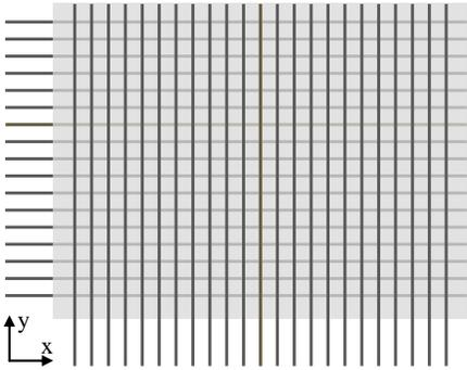
**Fig. 1:** Principle of electrode rows and columns.
