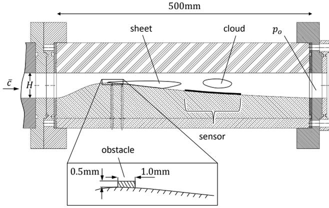
**Fig. 2:** Geometry of the convergent-divergent nozzle.
