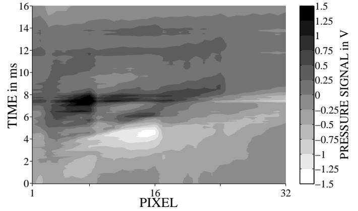
**Fig. 5:** Pressure signal history of all 32 pixels during one cloud cycle corresponding to the high-speed photographs shown in Fig. 4.
