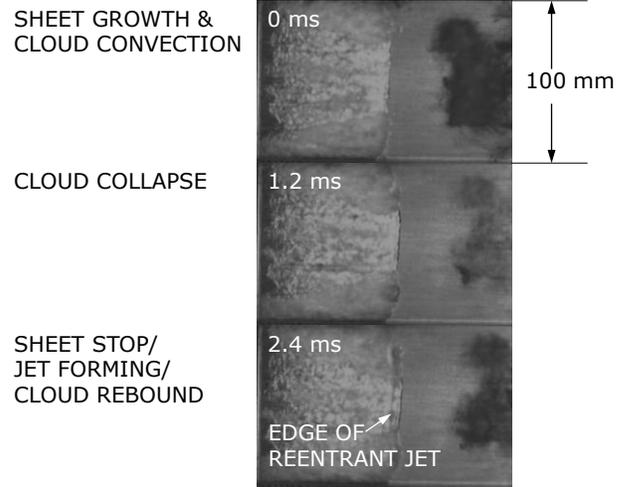
**Fig. 4:** Forming of the reentrant jet triggered with the cloud collapse operating point for  $Re = 110e3$  and  $\sigma = 5.4$ .
