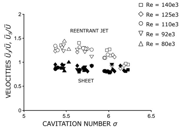
**Fig. 5:** Velocities of the reentrant jet and the sheet growth for the cloud regime. Note: The velocities are time averaged for the spreading and the sheet growth phase.
