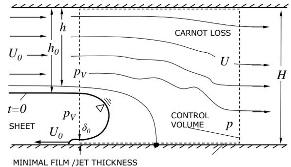
Fig. 11: Control volume for the momentum balance to determine the initial film thickness at  $t=0$ .
