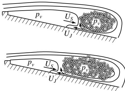
Fig. 6: Reentrant jet for  $Re = 75e3$  and  $\sigma = 5.7$
