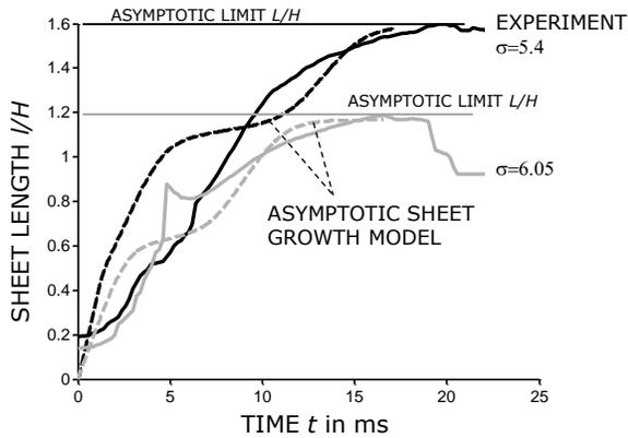
Fig. 8: Comparison of the sheet model and experimental results for  $Re = 140e3$ .
