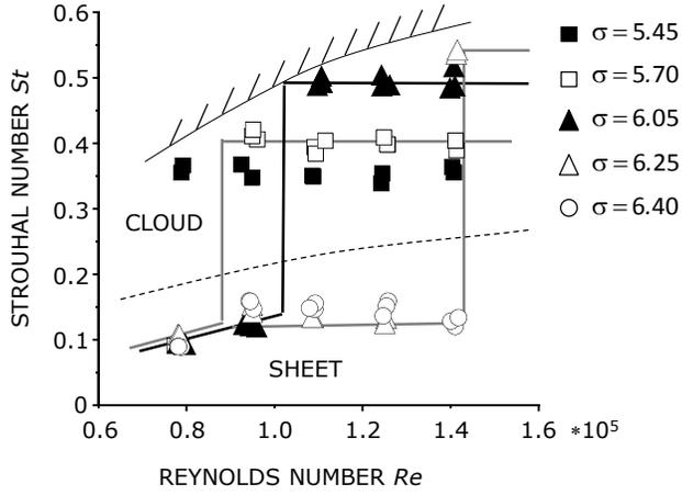
**Fig. 1:** Transition from sheet to cloud cavitation for the nozzle shape described by Keil, Pelz, Ludwig [1].
