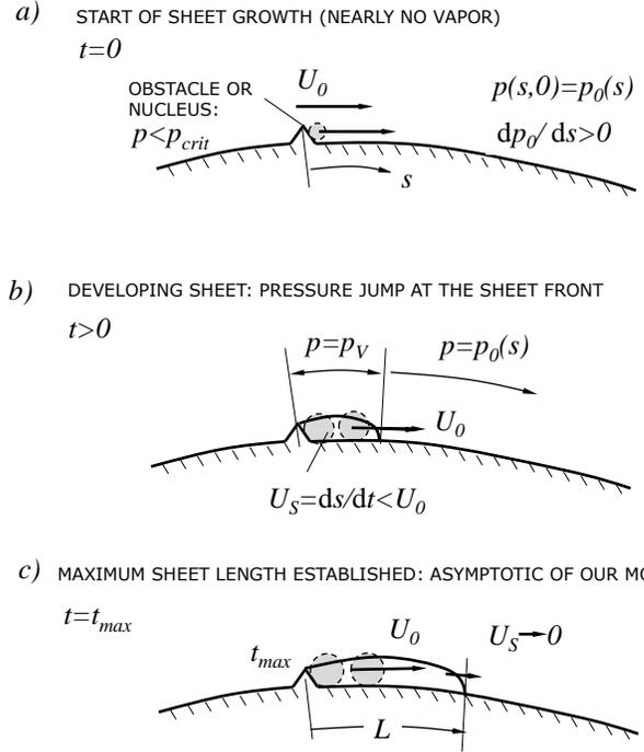
Fig. 7: Asymptotic sheet growth model. a) Growing of a nucleus at  $s=0, t=0$ ; b). Sheet growth by continuous feeding the sheet by cavitation bubbles traveling with the outer velocity. The bubbles are subjected to the described pressure distribution and follow the RPE. The sheet velocity is smaller than the feed velocity! c) Asymptotically the sheet comes to a rest, as soon as the bubble reaching the sheet front growths unstable.
