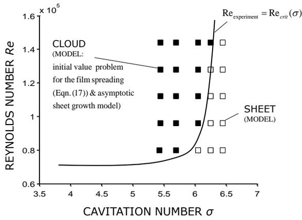
**Fig. 12:** Predicted stability map & comparison with the experimental stability limit (see Fig. 3 for the experimental results).
