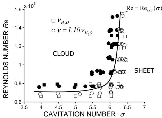
**Fig. 3:** Stability map: Experimental determined critical Reynolds  $Re = Re_{crit}(\sigma)$  number for the transition from sheet to cloud cavitation for two viscosities.
