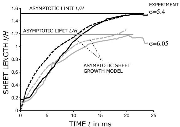
Fig. 9: Comparison of the sheet model and experimental results for  $Re = 110e3$ .
