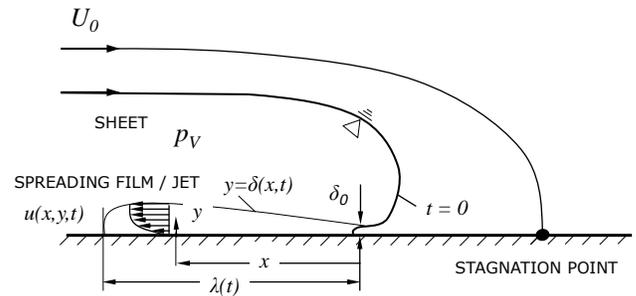
Fig. 10: Reentrant jet considered to be a spreading viscous film.
