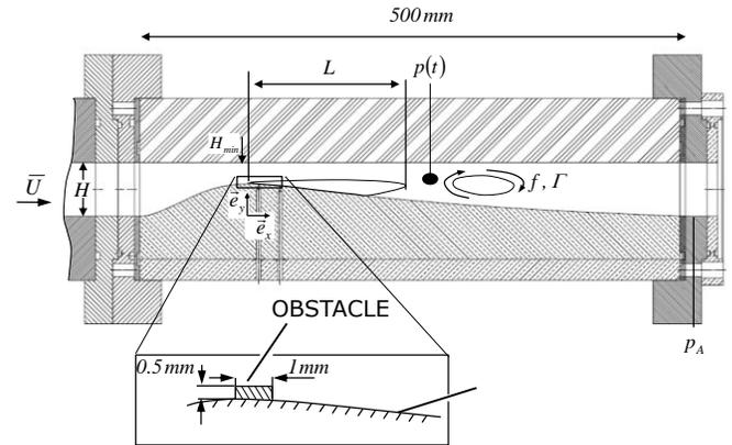
**Fig. 2:** Nozzle geometry adapted in a close loop test bench at the chair of Fluid Systems Technology - Technische Universität Darmstadt.
