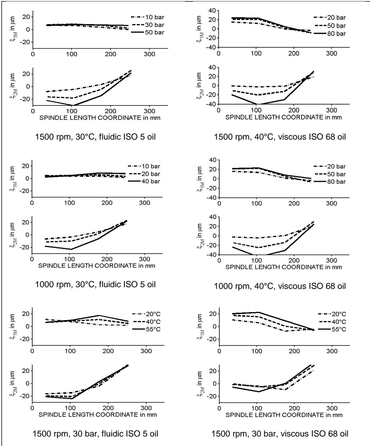
Figure 7: Idle spindle bending lines for various operation points
