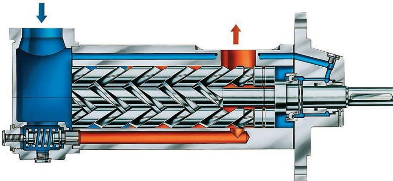
**Figure 1:** 3-spindle screw pump /8/
