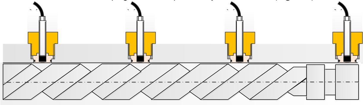
Figure 5: Axial sensor positions
