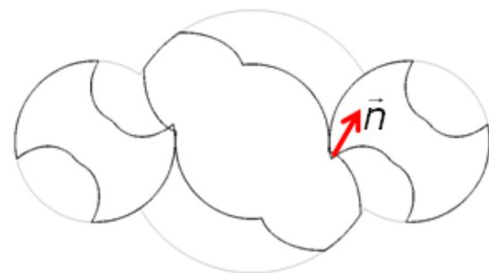
Fig. 8: Hertz contact model.
