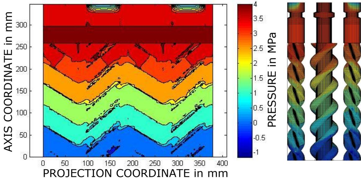
**Figure 4:** pressure deviation in standard operation point
