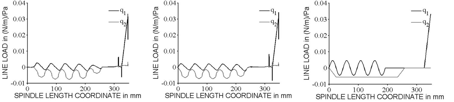
**Figure 7:** Line load diagrams for  $\varphi = 0^\circ$  and  $\varphi = 90^\circ$  and simplified for bending line model
