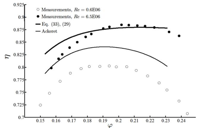
Fig. 4 Comparison of efficiency scale-up using Eq. (33) and (29)
