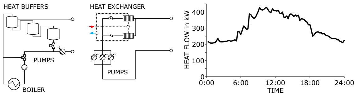
**Figure 1:** Left: Hydraulic diagram of the Boiler circuit. Middle: District heating circuit. Right: Average daily load cycle.
